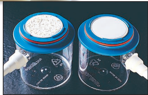
Spallation debris collected onto a microporous filter membrane after recirculating water for 48 hours through TPE tubing (left) and STA-PURE tubing (right).
